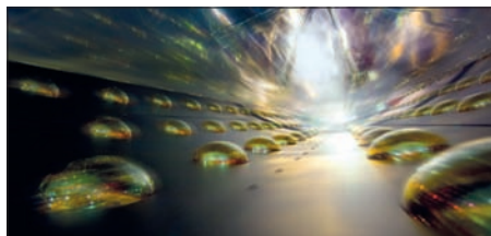
The sensitive photomultiplier tubes, which line the Daya Bay detector walls, are designed to amplify and record the faint flashes that signify an antineutrino interaction. (Image credit: Roy Kaltschmidt/Lawrence Berkeley National Laboratory.)
